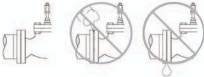
Fig. 3. Piping must prevent leakage.
