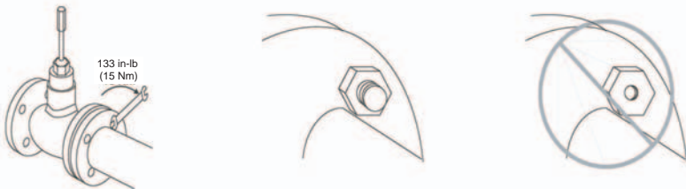
Fig. 4. Basic proper bolt length.
